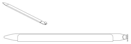
Figure 41. Optical transceiver (SFP, SFP+, and XFP) extraction tool
